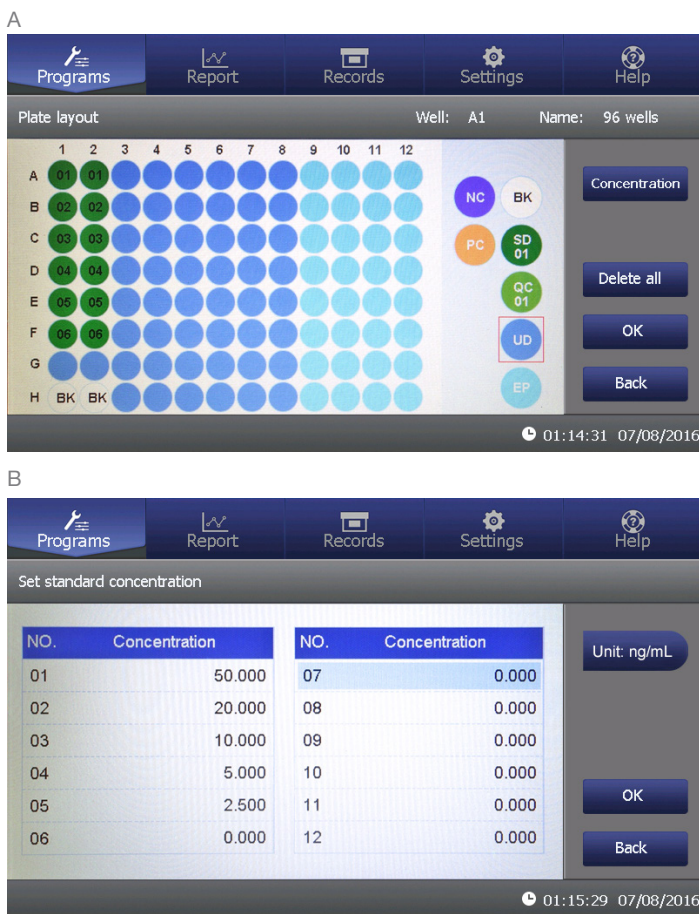
Figure 2. Setting up the plate and assigning standard values using the Ao software. A) The plate layout interface set to designate where the standards, blank wells, and unknowns are located. Each sample was loaded in duplicate. B) Standard concentration values and units (as provided by manufacturer) were entered into the system in order to generate a standard curve and interpolate sample values.
